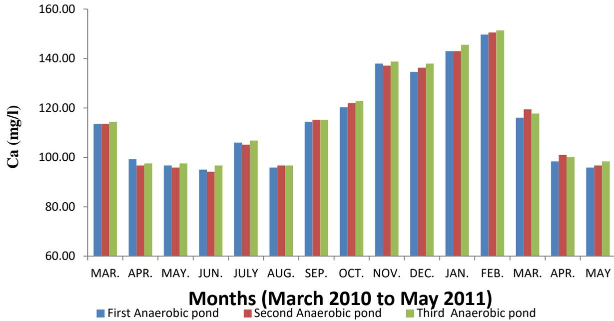
**Fig. 5. Ca (Calcium) in three anaerobic sewage stabilization ponds, Bikaner.**
