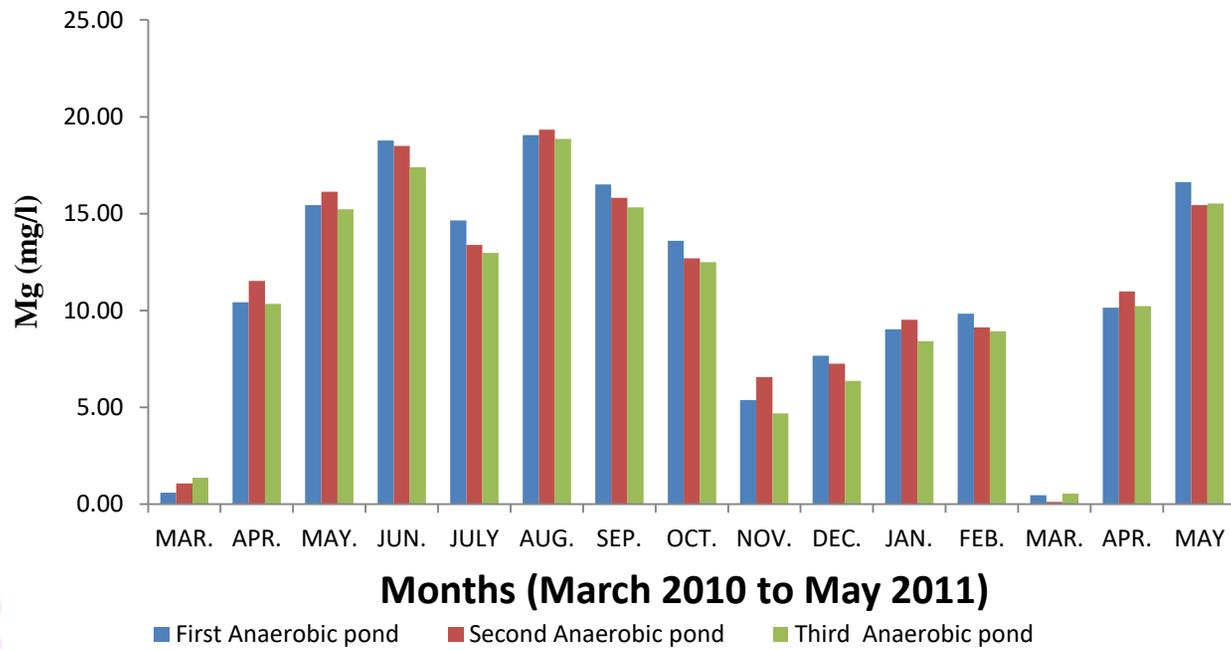
**Fig. 7. Mg (Magnesium) in three anaerobic sewage stabilization ponds, Bikaner.**
