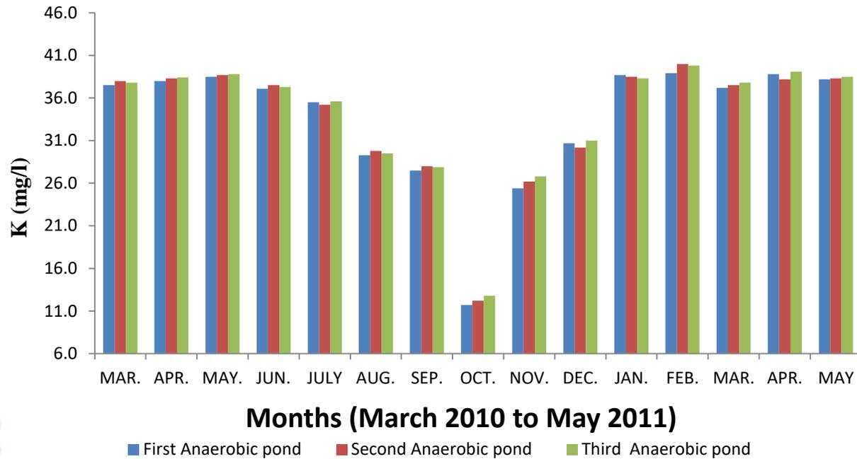
**Fig. 3. K (Potassium) in three anaerobic sewage stabilization ponds, Bikaner.**
