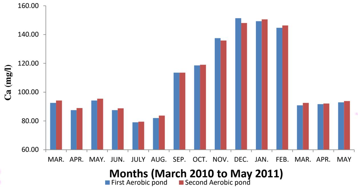
**Fig. 6. Ca (Calcium) in two aerobic sewage stabilization ponds, Bikaner.**
