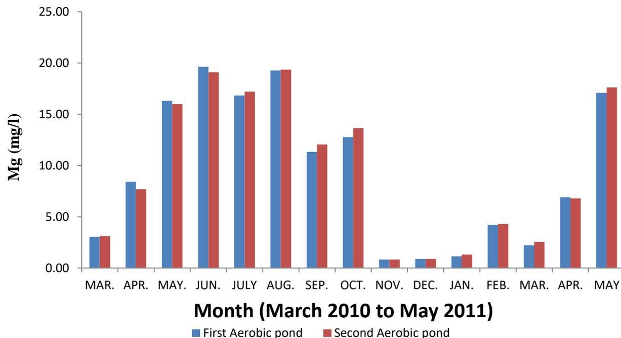
**Fig. 8. Mg (Magnesium) in two aerobic sewage stabilization ponds, Bikaner.**
